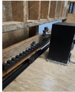
Figure 6. Motor Gear Rack
