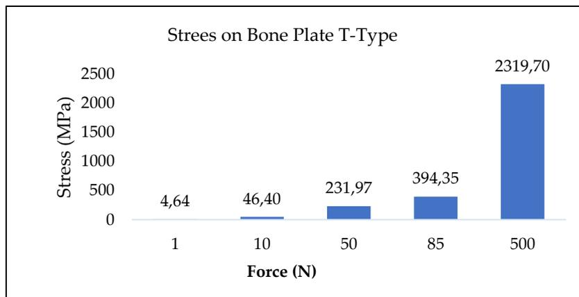
**Figure 3** Stress in T-Type Bone Support
