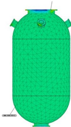
**Figure 2** Finite Element Analysis on a Biodiesel Reactor
