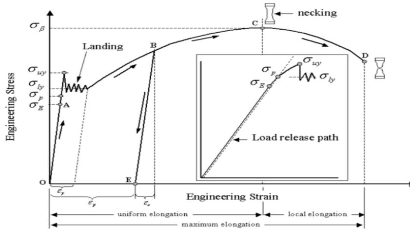
**Figure 1** Material Behavior Under Tensile Force
