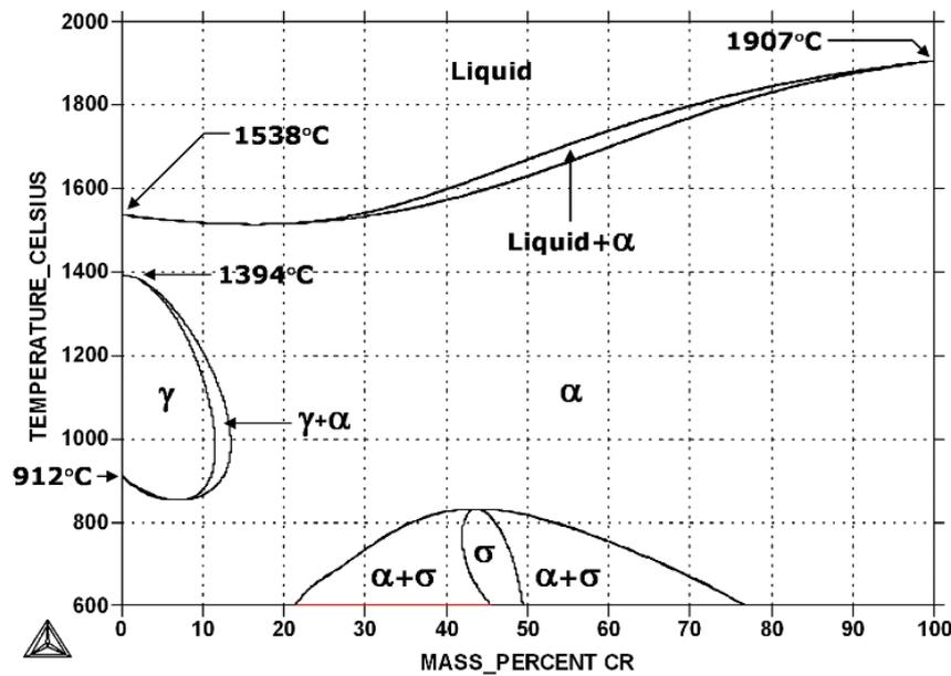
Figure 5 Stainless Steel Phase Diagram
