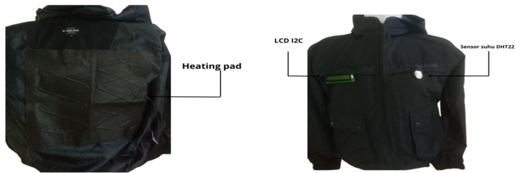
Figure 6. The jacket with installed system
