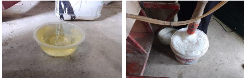
Gambar 1 Sika foam agent (a) bahan baku foam agent (b) buih foam agent
